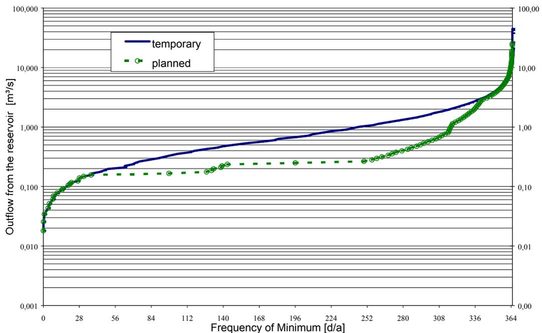
Fig. 3: Example of the simulation of the frequency of minimum outflow from the reservoir in the area of the planned dam
