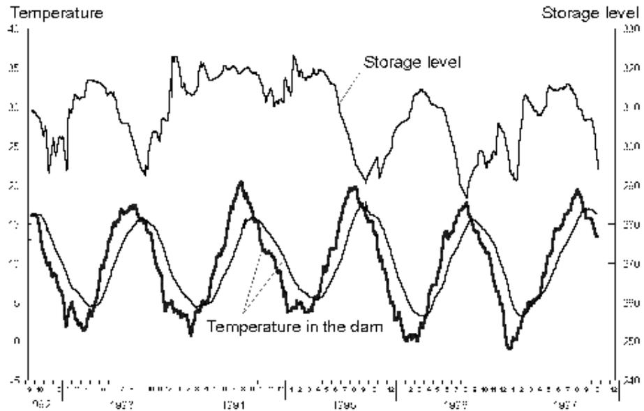
**Fig. 16: Storage Level and Masonry's Temperature in the Area of the Dam's crest**
