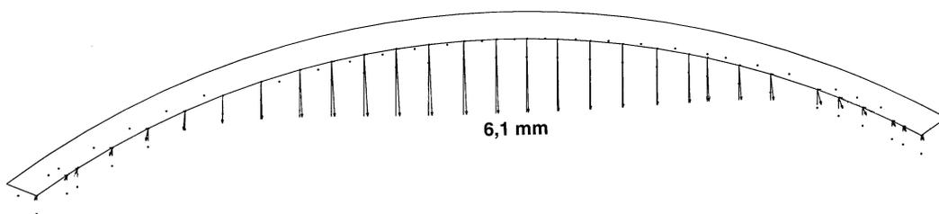
**Fig. 14: Stability Analysis: Rise of Storage Level from 295 mNN to 315 mNN, Displacements caused by Rise of Storage Level, Top View on the Dam's Crest**
