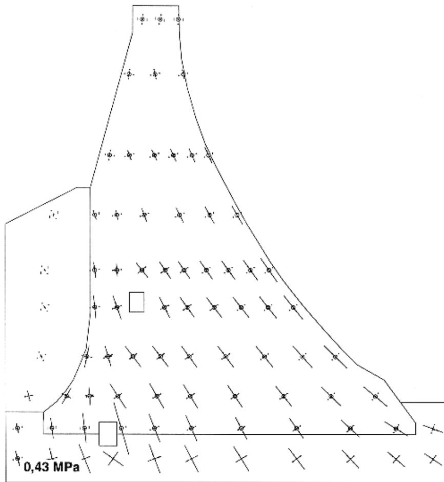
**Fig. 15: Stability Analysis: Rise of Storage Level up to 322,5 mNN, Principal Normal Stresses in Valley Midth**
