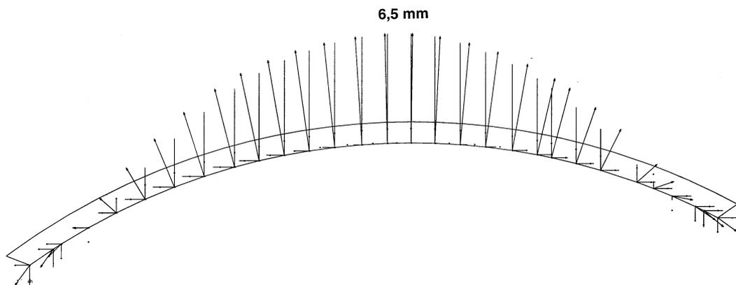
**Fig. 20: Stability Analysis: Displacements at the Dam's crest caused by Temperature Rise from Winter to Summer**
