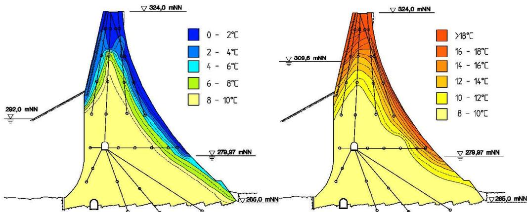
**Fig. 17: Temperature Distribution in the Dam during Winter**
