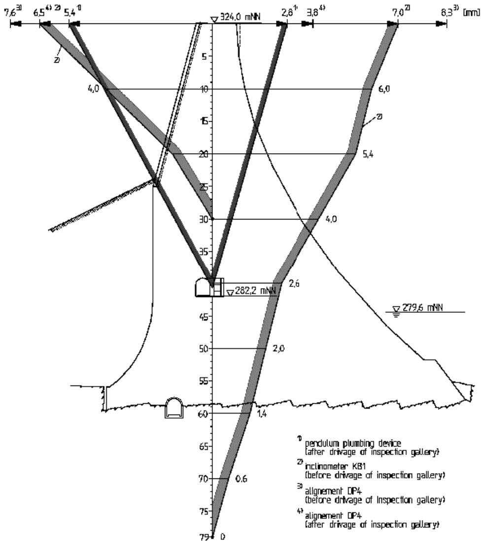
**Fig. 11: Displacements of the Dam in Valley Midths caused by a Raise of Storage Level from 295 mNN to 315 mNN and by a temperature increase of 10° C**
