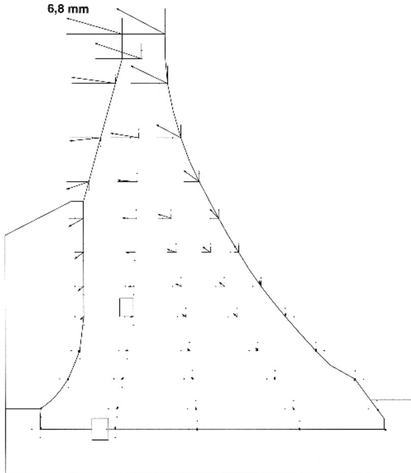
**Fig. 19: Stability Analysis: Displacements in Valley Midth caused by Temperature Rise from Winter to Summer**
