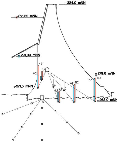
**Fig. 9: Pore Water Pressure Measurements MQ VI**
