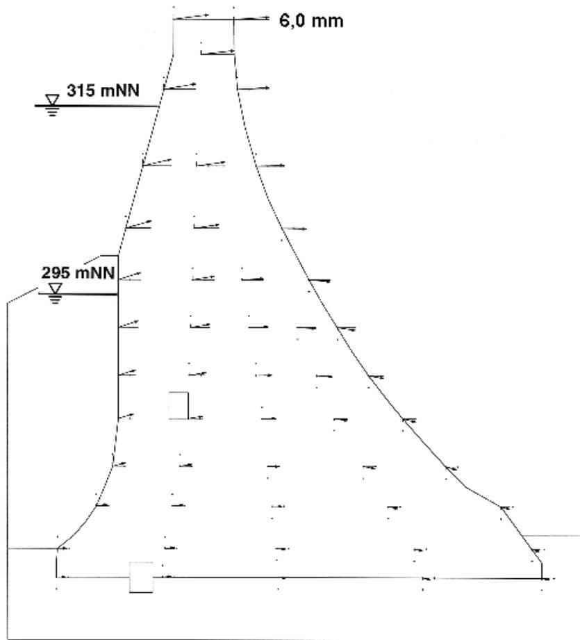
**Fig. 13: Stability Analysis: Rise of Storage Level from 295 mNN to 315 mNN, Displacements caused by Rise of Storage Level**
