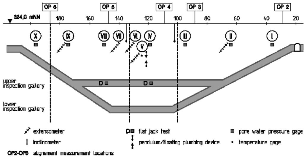
Fig. 2: Measuring Devices and Locations (Longitudinal Section)
