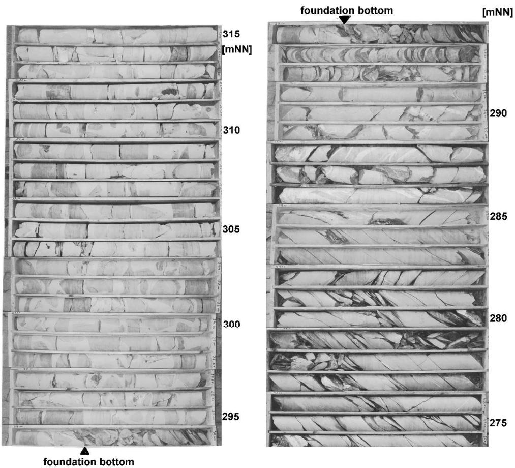
Fig. 5: Drill core KB 7 (masonry)
