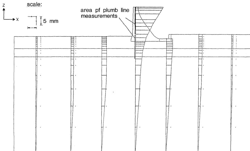
Fig. 8: Horizontal displacements due to raising the storage level from 217 to 241 m above MSL
