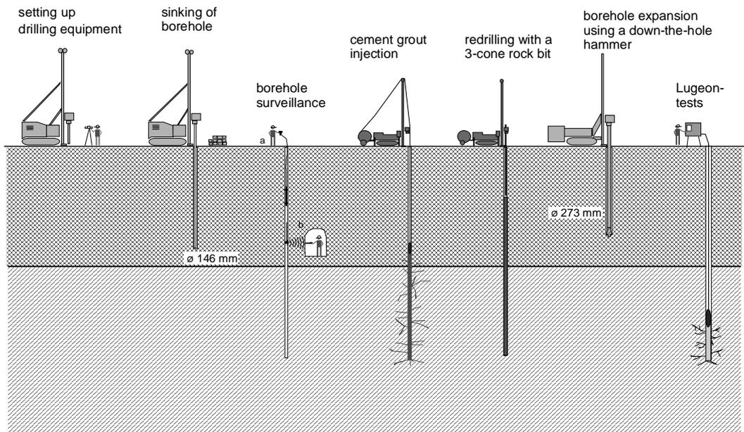
Fig. 15: Borehole procedure as a preparation for the prestressed anchors
