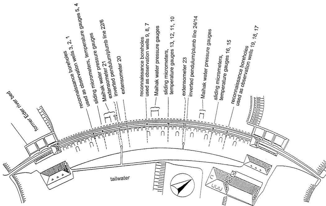
Fig. 4: Dam plan with measuring devices in cross-sections
