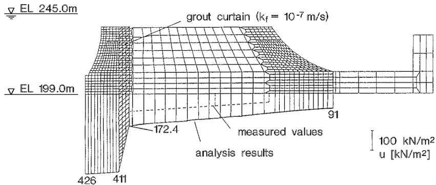
Fig. 11: Seepage analysis: Distribution of water pressure in the dam foundation area
