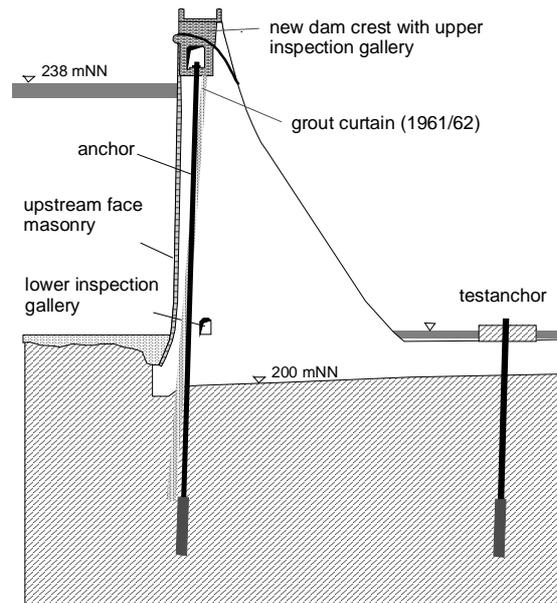
Fig. 3: Cross-section of the dam
