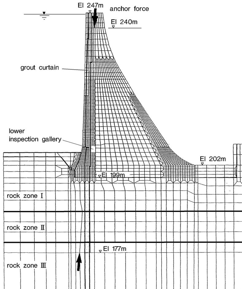
Fig. 5: Detail of the 2D finite element mesh
