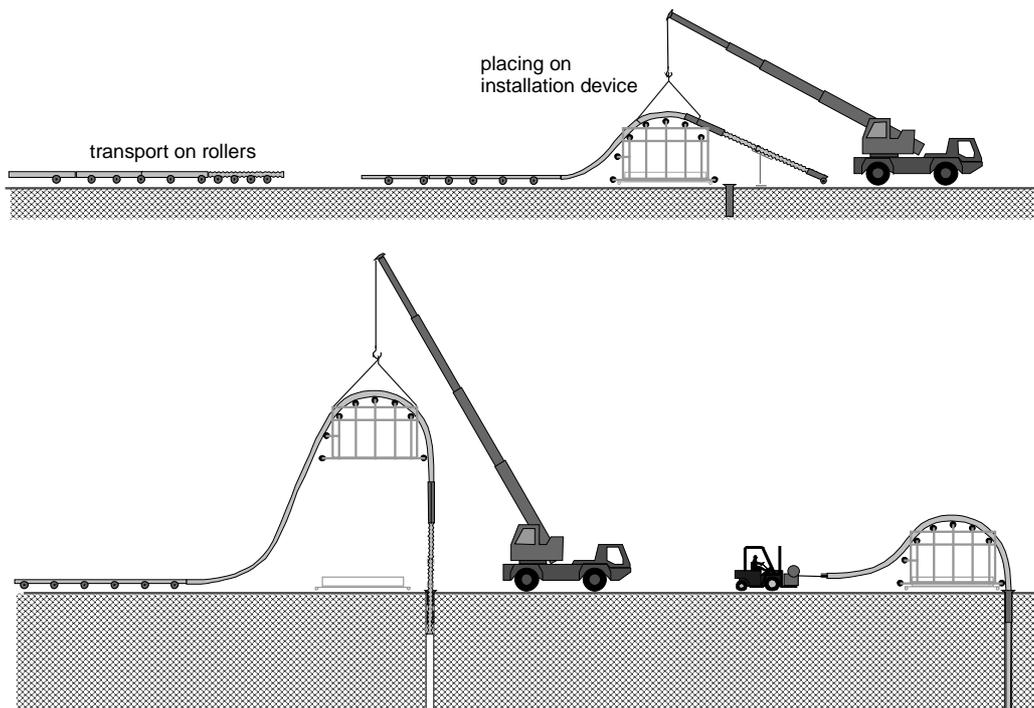
Fig. 18: Anchor transport and installation
