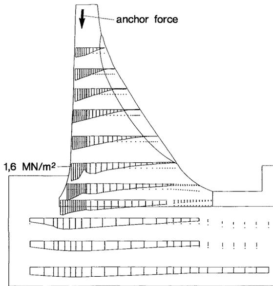
Fig. 9: Vertical stresses due to dead weight and anchor forces
