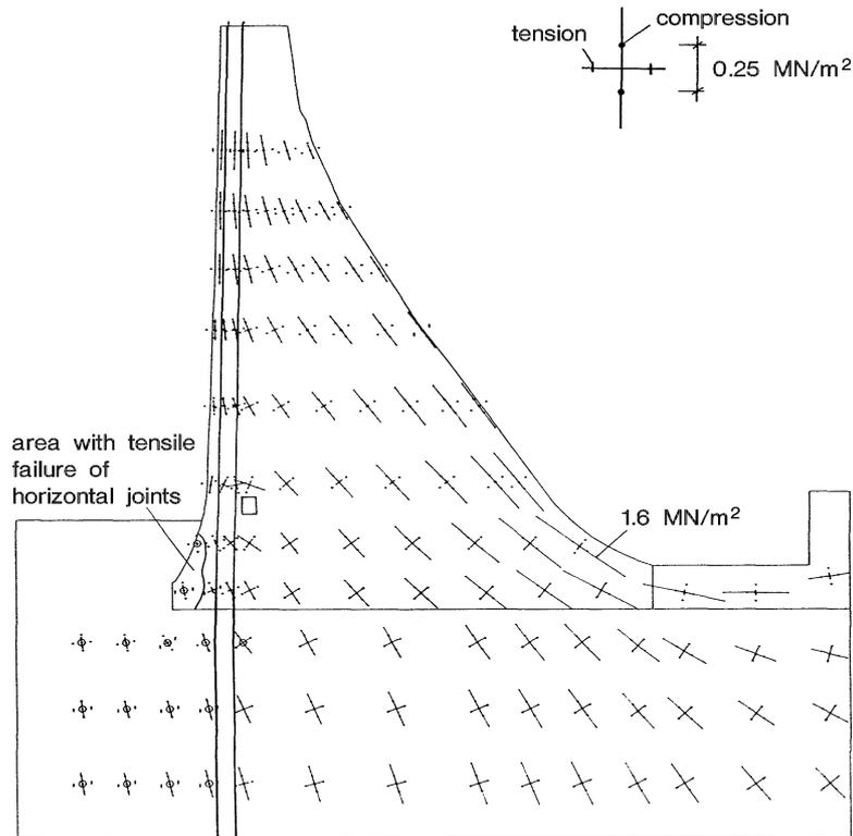
Fig. 12: Principal normal stresses: dead weight, anchor forces, storage level at el. 246,85 m
