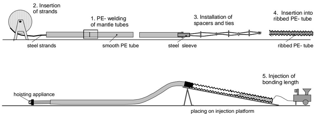
Fig. 17: Anchor manufacturing scheme
