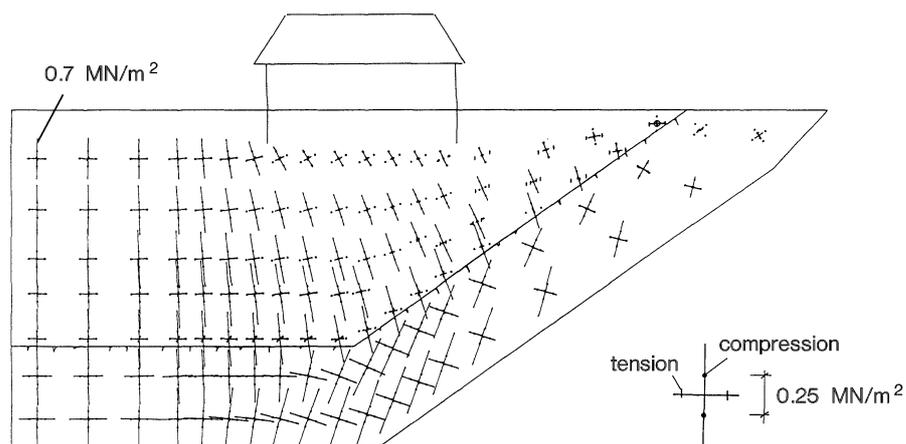
Fig. 14: Principal normal stresses: dead weight and anchor forces, longitudinal section on the upstream side of the wall
