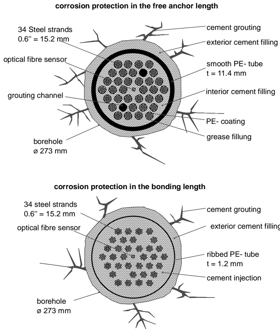
Fig. 16: Anchor cross-sections
