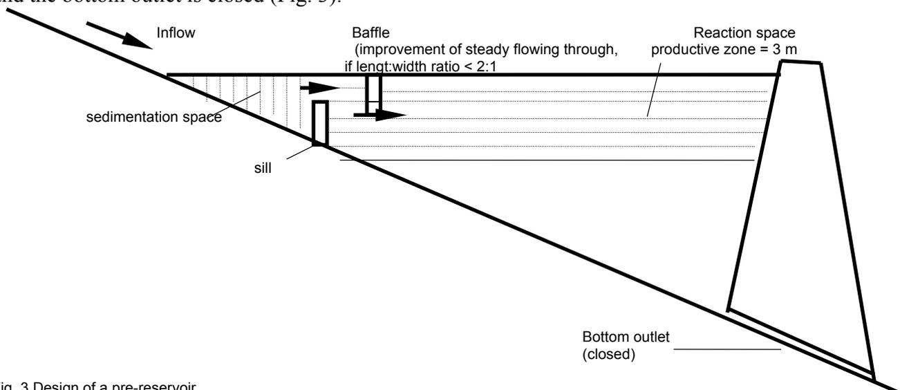
Fig. 3 Design of a pre-reservoir
