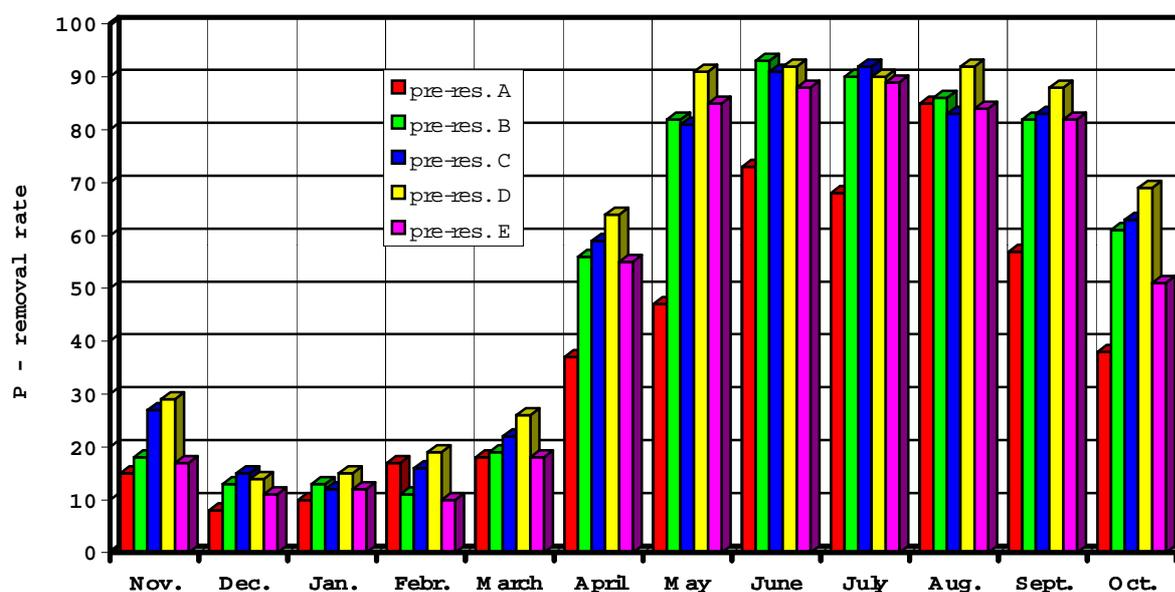
Fig. 4 P-removal rate of the pre-reservoirs of the Eibenstock dam (orthophosphate-P)
