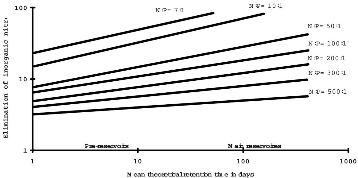
Fig. 2 Empirical estimation of the removal of inorganic nitrogen by reservoirs in dependence on
