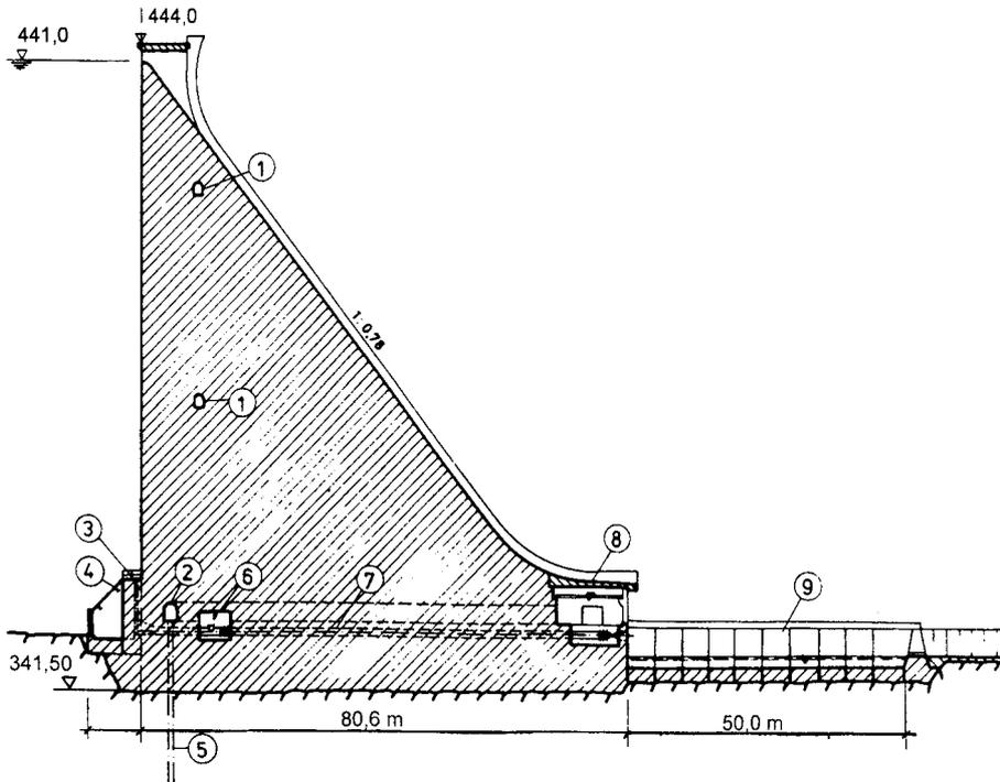
Fig.:4 Cross section gravity dam
