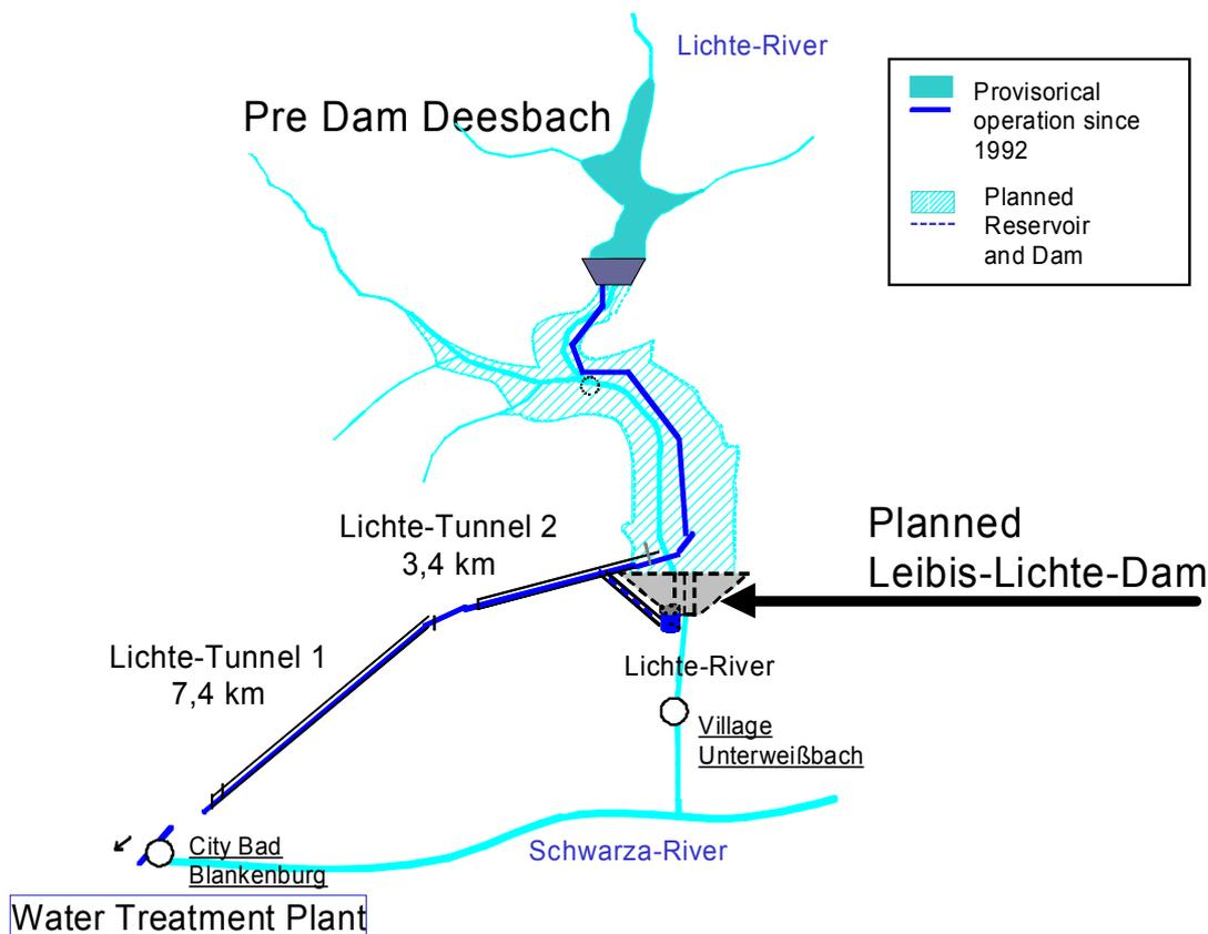
Fig.:6 Schematic view of the water collection system Leibis-Lichte
