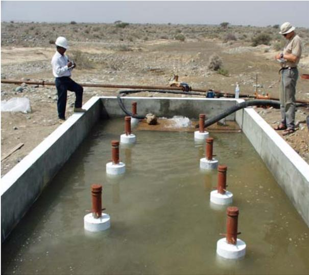
fig. 2 Infiltration test basin during the execution of a test
