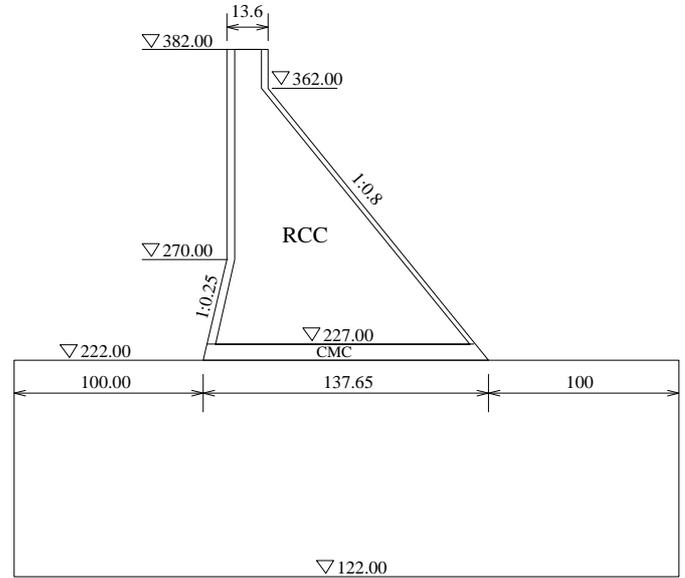
Fig. 2 Non-overflow section of Longtan RCC
