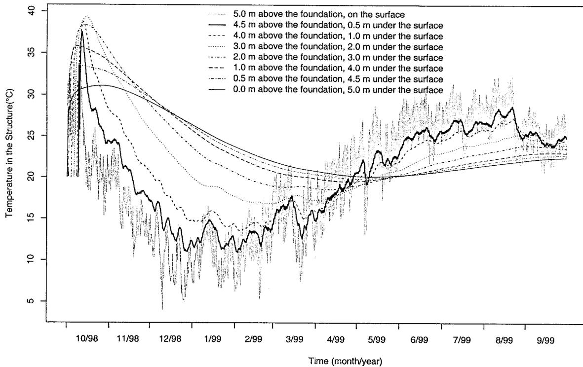
Fig. 5 Temperature Change at Different Locations During the First Year after the Completion of the Concrete Placement
