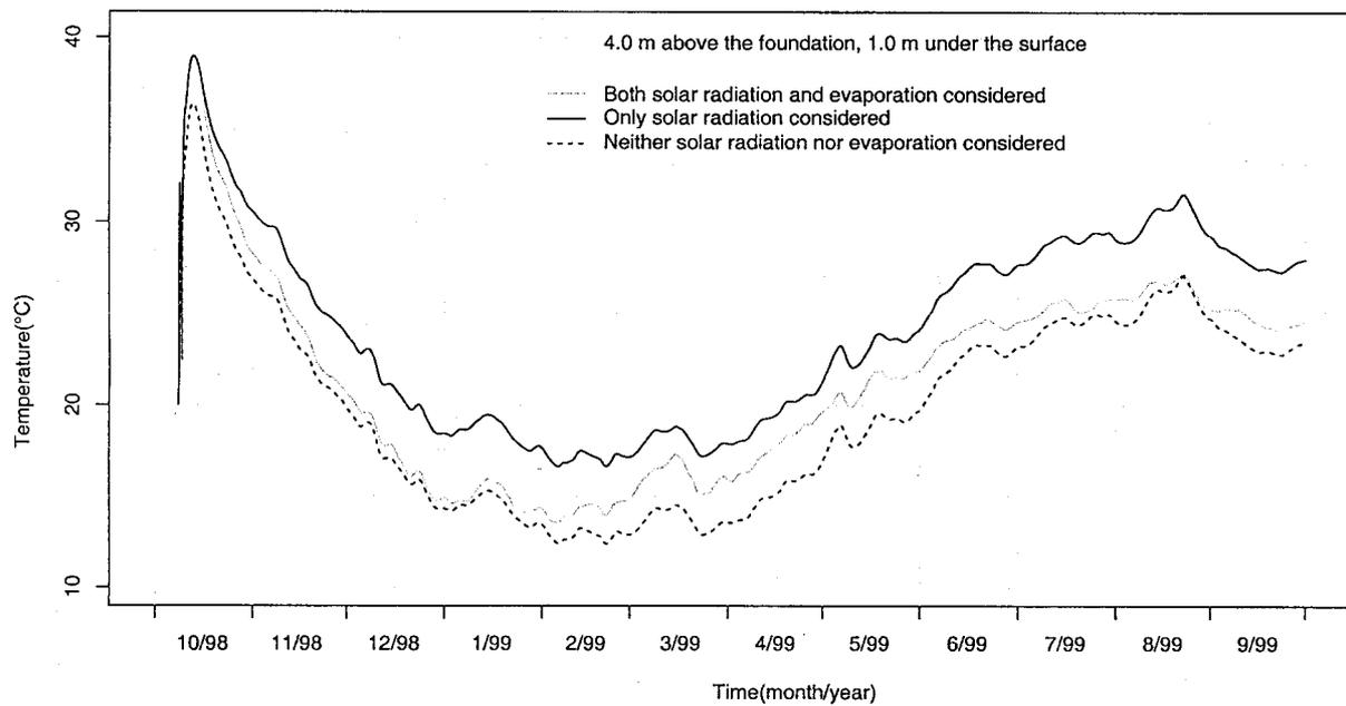
Fig. 7 Comparison of Temperature Development Calculated under Different Conditions
