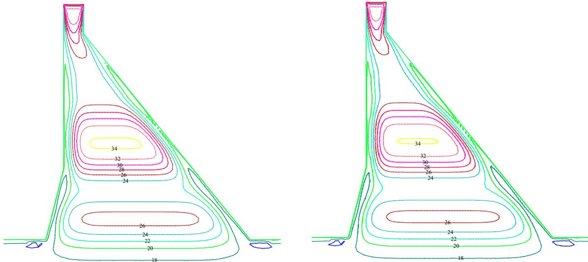
Fig. 4 Isothermal Lines of Longtan RCC Dam at the Completion of Concrete Placement, Calculated with TESAR using the Conventional Method (left) and the New Method (right)
