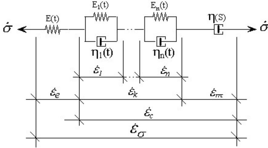
**Fig. 1 Stress Related Strain Components**
