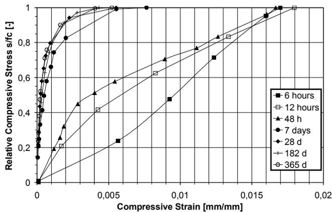
Figure 2. Comparison of typical stress-strain-curves at different RCC ages.
