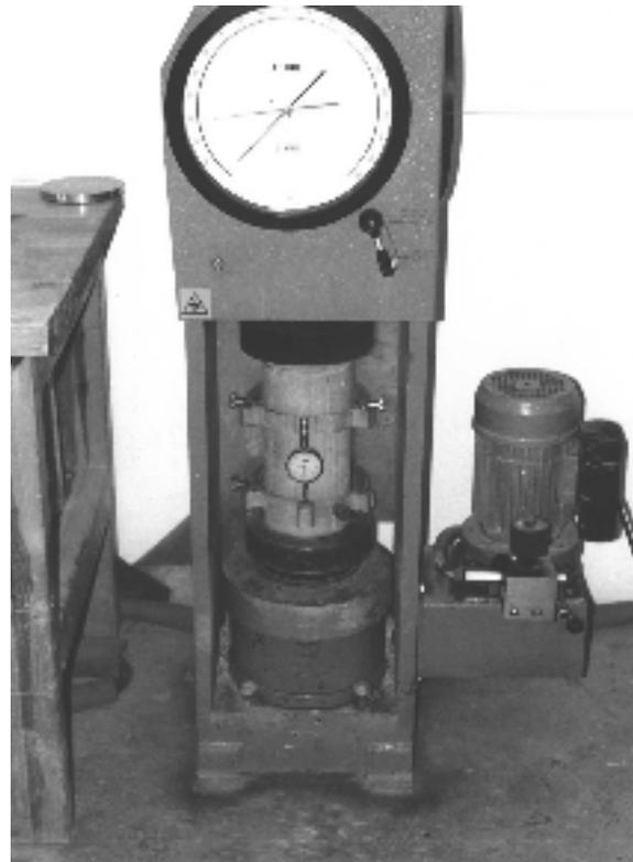
Figure 1. Setup of static elastic modulus test.
