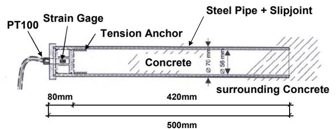
Figure 4. Longitudinal section of stressmeter.
