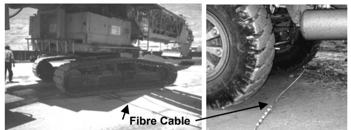
Figure 2. Fibre cable impacts due to on-site equipment.
