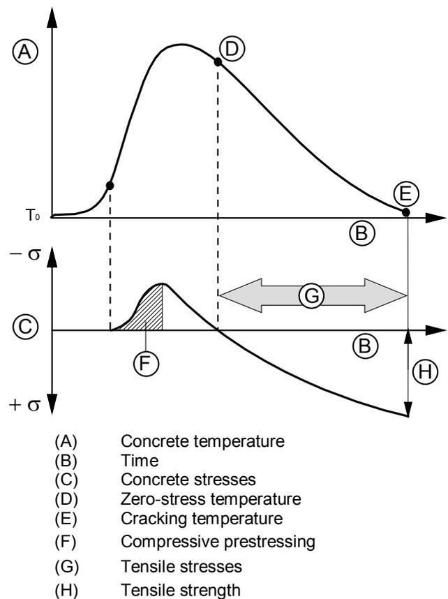
Figure 1. Stresses in young concrete under restrained deformation.
