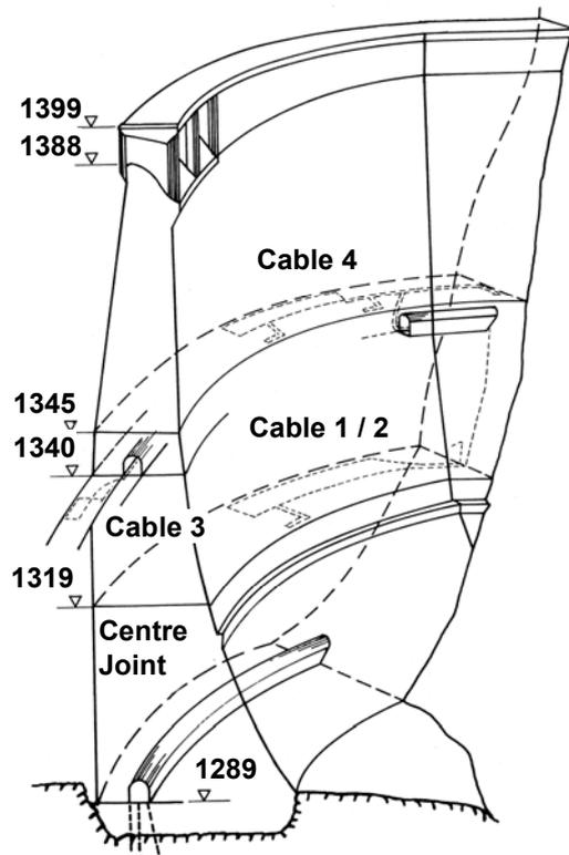
Figure 10. Isometric illustration of Shimenzhi Arch Dam.
