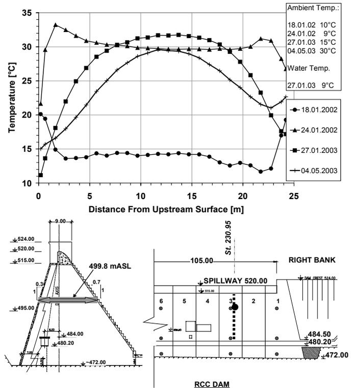
Figure 7. Wala Dam: Selected temperature profiles at block 3, elevation 499.8 mASL.
