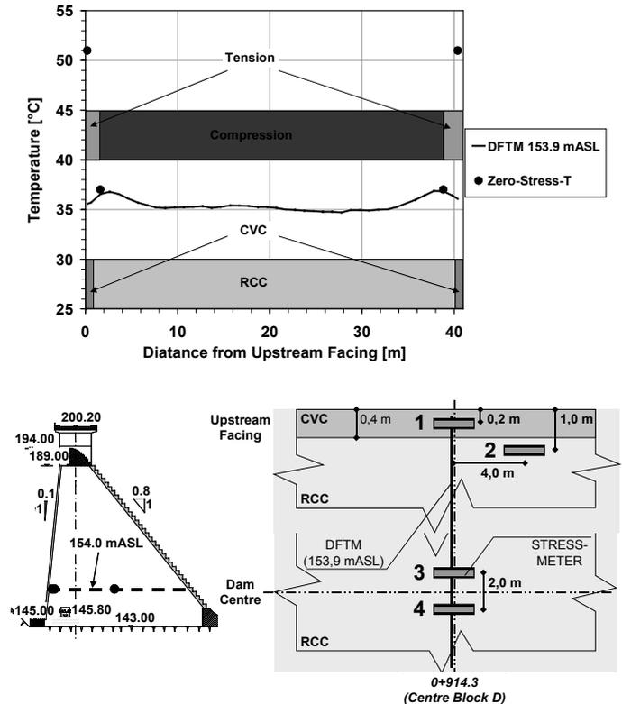
Figure 9. Mujib Dam: Zero-stress-temperature distribution and DFTM at the centre of block D, elevation 154.0 mASL.
