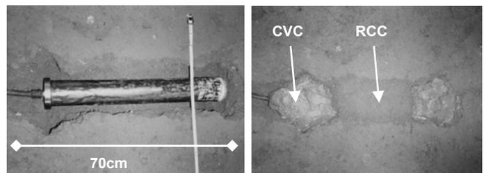
Figure 5. Installation sequence of stressmeters in RCC.
