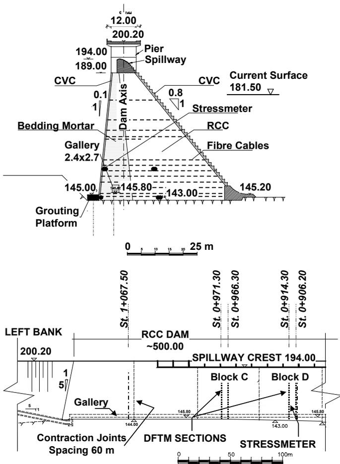
Figure 8. Mujib Dam: Cross section and longitudinal section of the left bank.
