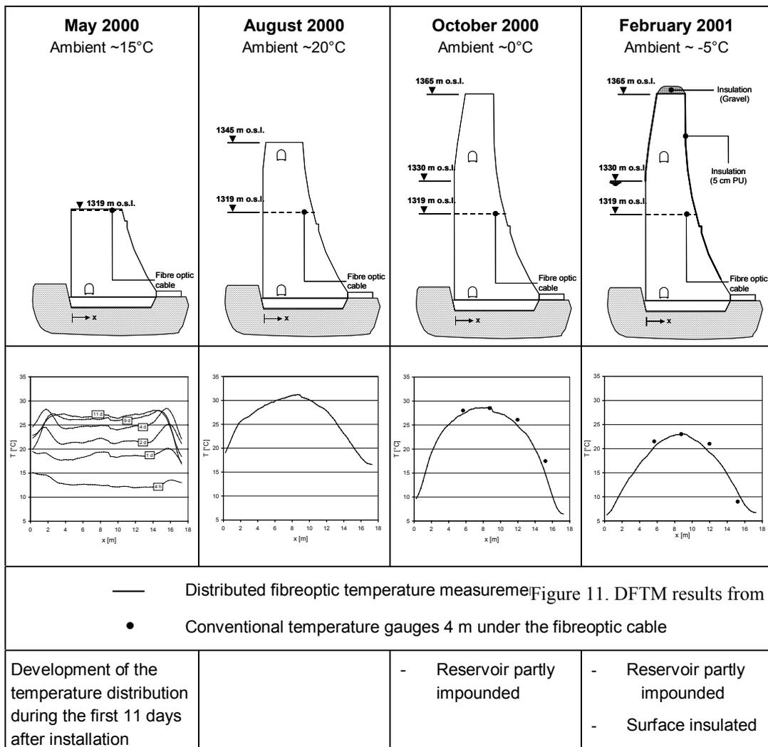
Figure 11. DFTM results from Shimenzhi Arch Dam.
