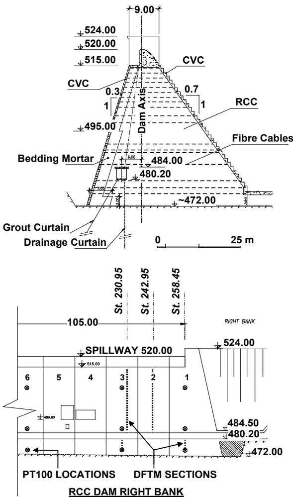
Figure 6. Wala Dam: Cross section and longitudinal section of the right bank
